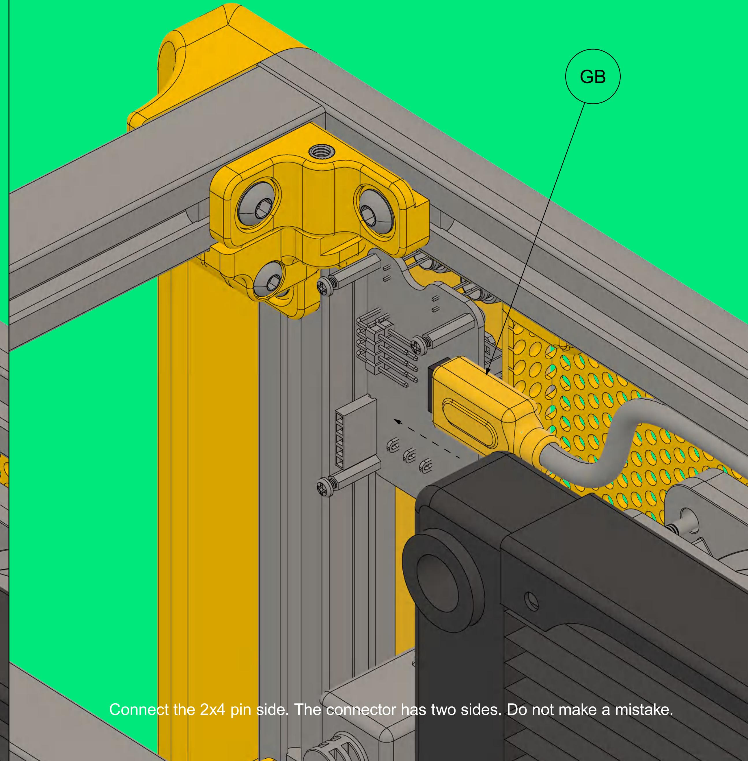
Connect the 2x4 pin side. The connector has two sides. Do not make a mistake.
