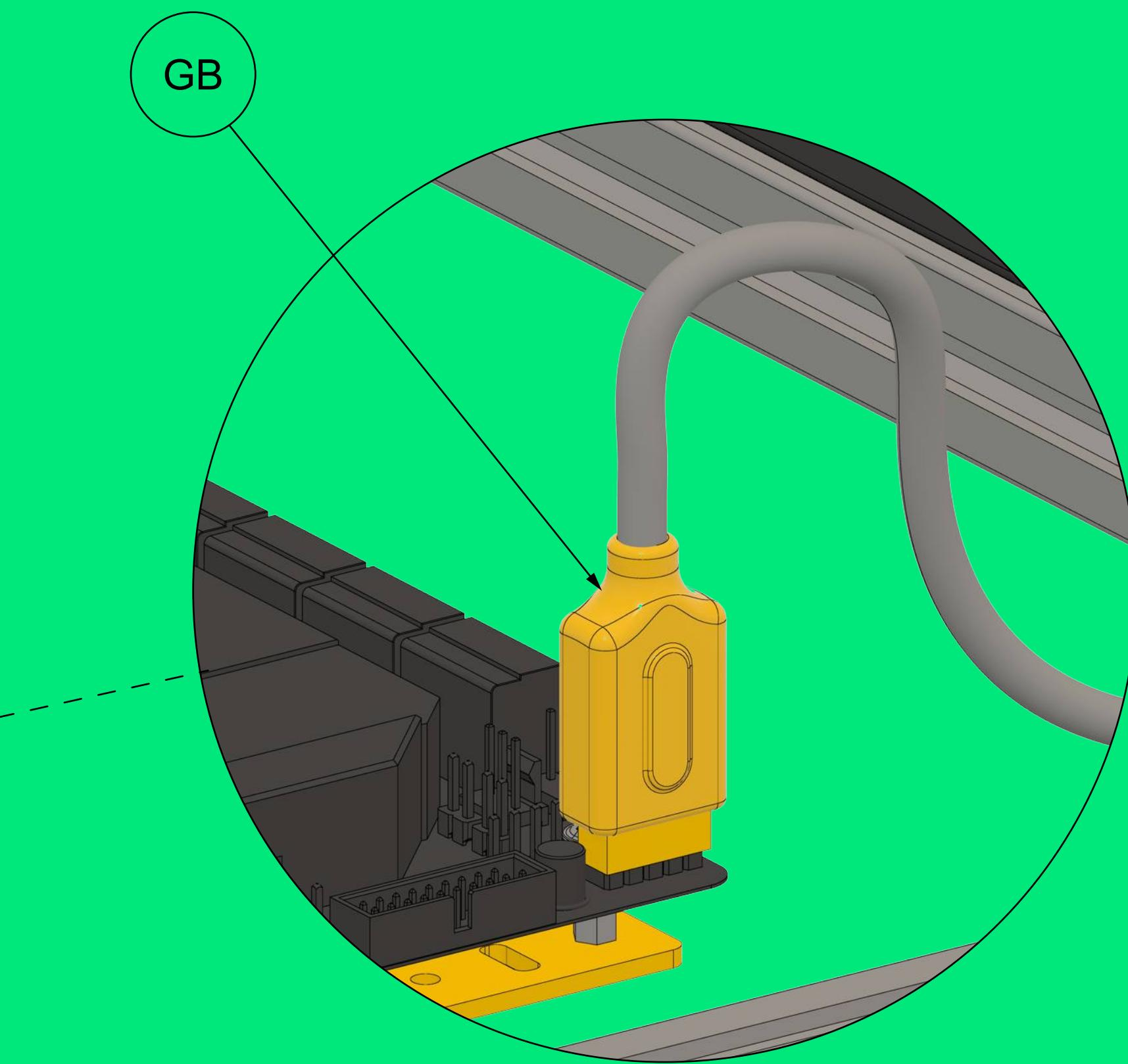
Connect the 2x5 pin side. The connector has two sides. Do not make a mistake.
