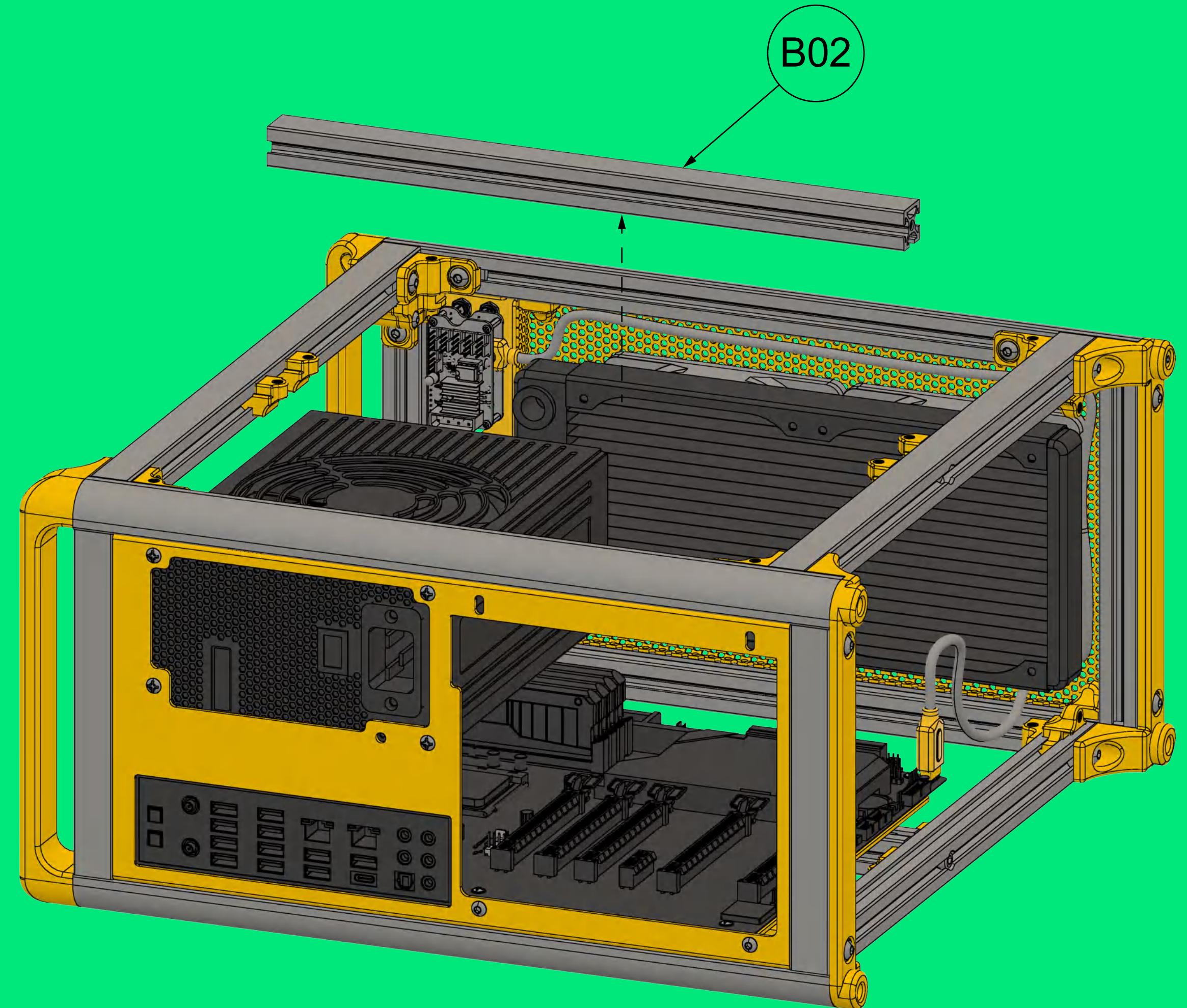
The aluminum frame must be removed once to connect the GPU.
